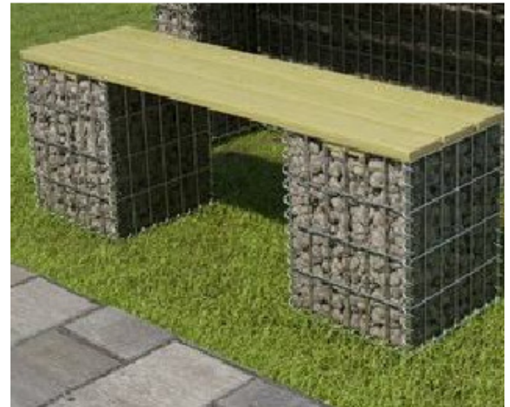
TYPICAL GABION SEAT NB: SUPPORT BASKETS TO BE FILLED WITH RECYCLED PLASTIC BOTTLES
