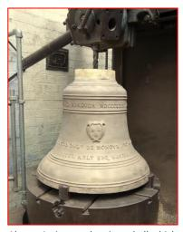
Above: An image showing a bell which has been sandblast cleaned, had its canons removed, and resin pad cast upon its crown to allow for a flat surface.
