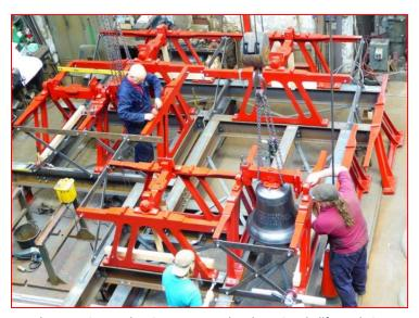
Above: An image showing a new steel and cast iron bellframe being erected in our works.
