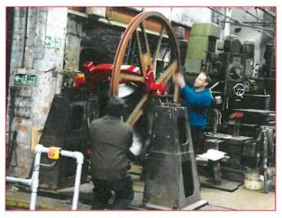
Above: An image showing a refurbished bell being swung in our testing stand.
