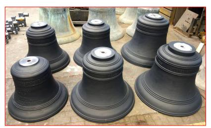
Above: An image showing a peal of bells which have been tuned, had their canons removed, had resin pads cast upon their crowns and have received their first coat of polish. Ready to receive their new bell fittings.
