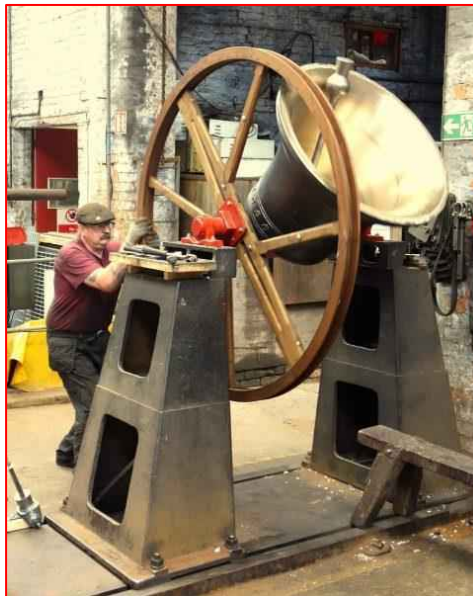
Above: An image showing a bell being swung and analysed in our testing stand.
